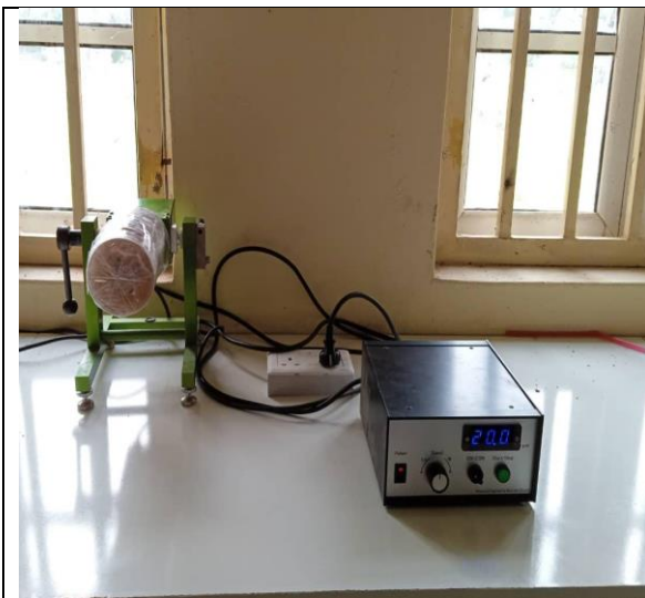
Plate 3A: Microgravity device setup with samples under zero gravity condition
